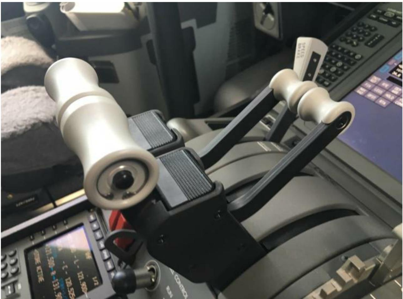
Autothrottle disconnect buttons on the side of the thrust lever and the reverse thrust levers on the right. Speedbrake lever at the back. (Photo by Charlie Page/The Points Guy)
