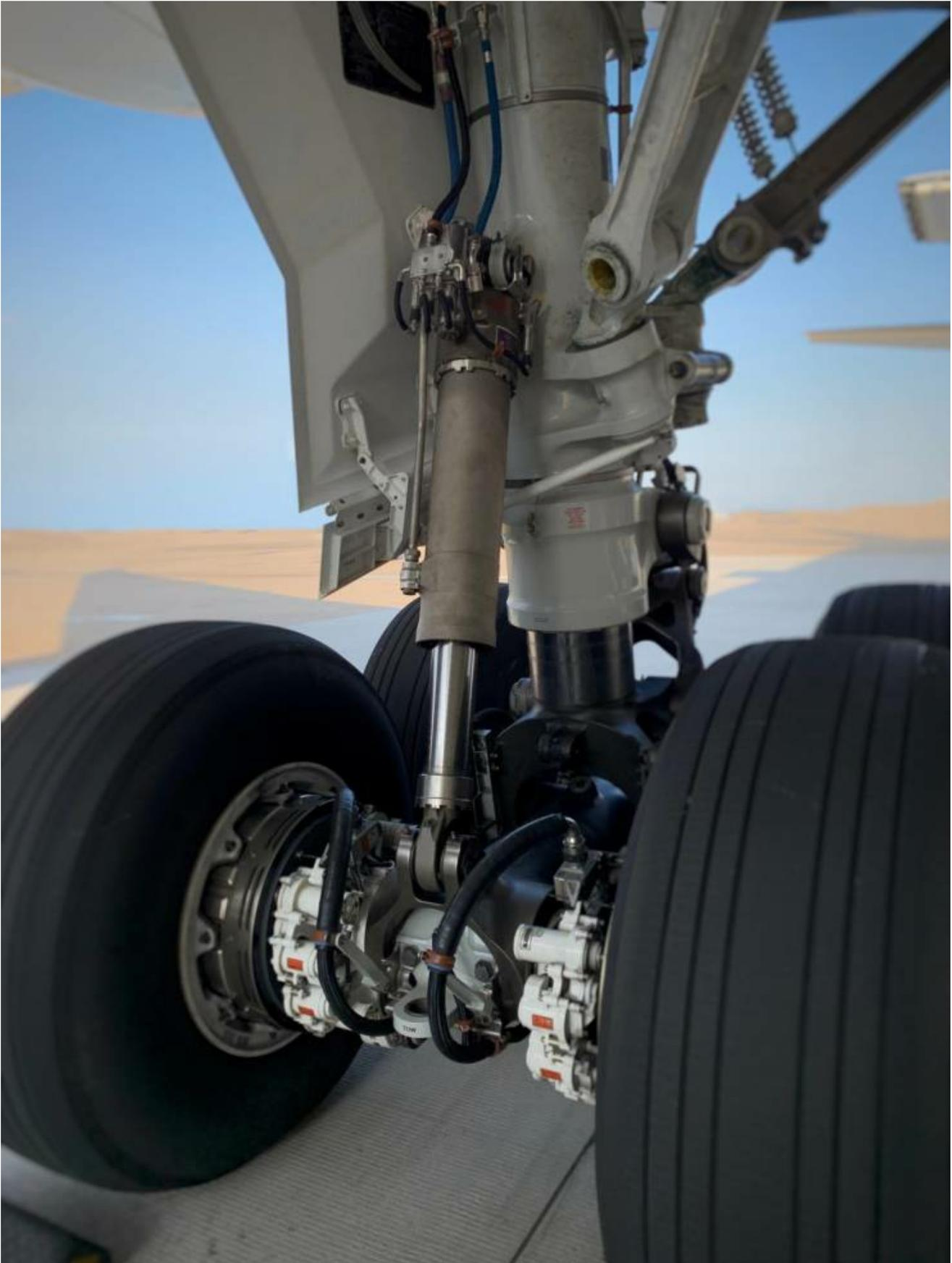
The hydraulic strut on the semi-levered gear of the 787-10. (Photo courtesy of 787 Guide)
