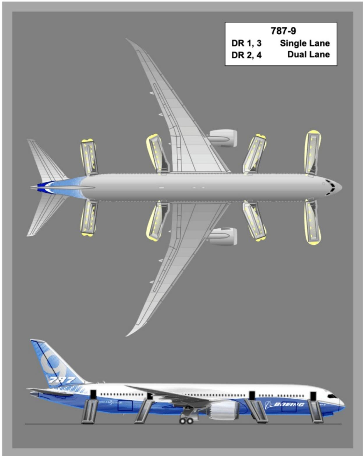
The doors and slide/rafts on the 787 Dreamliner. (Image courtesy of Boeing)
