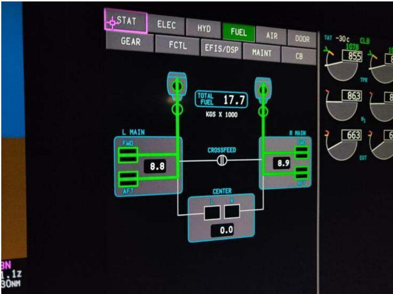
The fuel system on the 787 has a centre tank and a main tank in each wing. (Image Charlie Page/The Points Guy)
